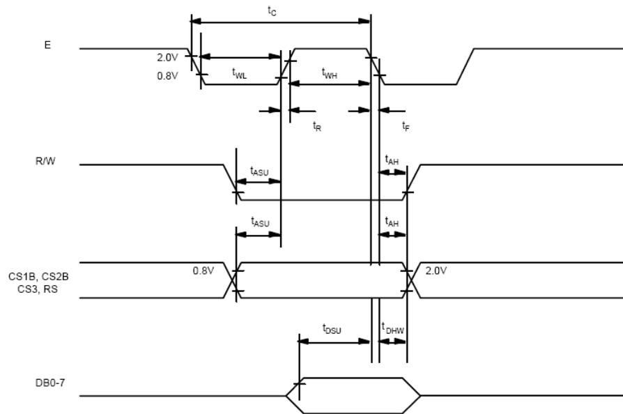
Figure 1. Write timing
