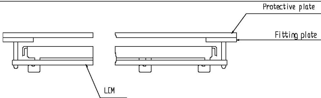
(2) When assembling the LCM into other equipment, the spacer to the bit between the LCM and the fitting plate should have enough height to avoid causing stress to the module surface, refer to the individual specifications for measurements. The measurement tolerance should be 0.1mm.
