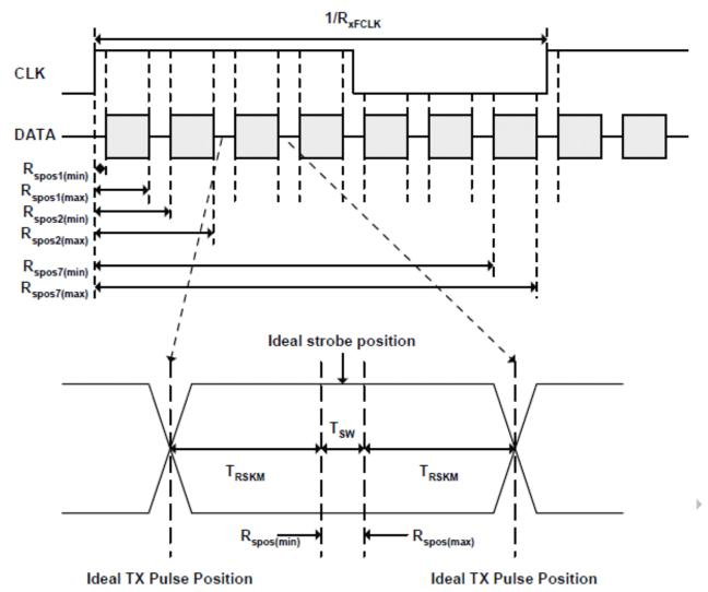
T<sub>RSKM</sub>: Receiver strobe margin R<sub>SPOS</sub>: Receiver strobe position
