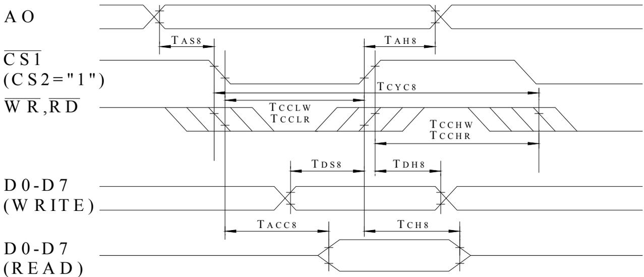
(V<sub>DD</sub>=3.3V, T<sub>A</sub>=25 )
