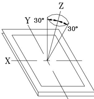
Inspection should be performed within  $\phi$  ( $\phi$  is usually  $30^{\circ}$ ) from Z axis to each X and Y axis. Inspection distance of any direction within  $\phi$  must be kept  $30 \pm 5$  cm to the display surface.
