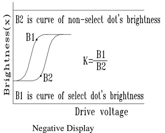
$$\text{Contrast Ratio (K)} = \frac{\text{Brightness of non-selected dot (B2)}}{\text{Brightness of selected dot (B1)}}$$
